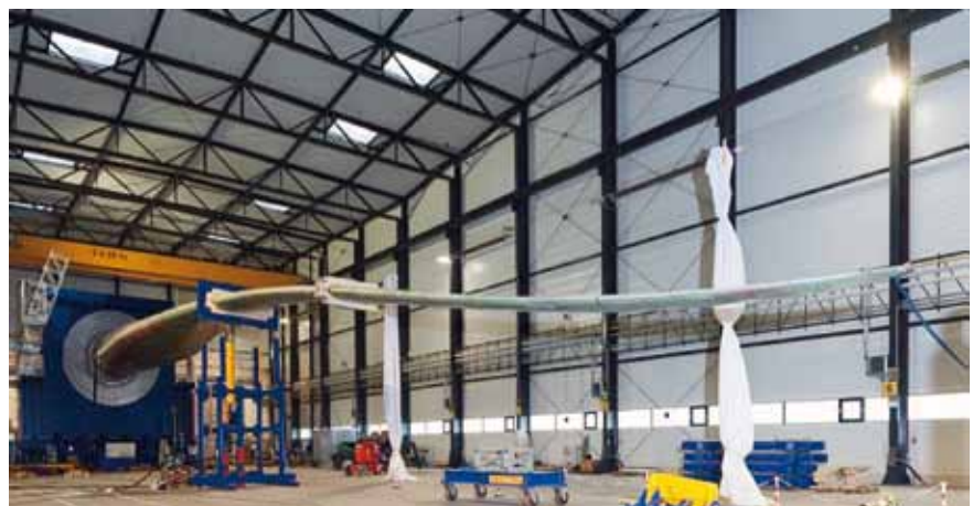
Figure 1: Testing of a large-scale rotor blade at the Fraunhofer Institute for Wind Energy Systems in Bremerhaven
