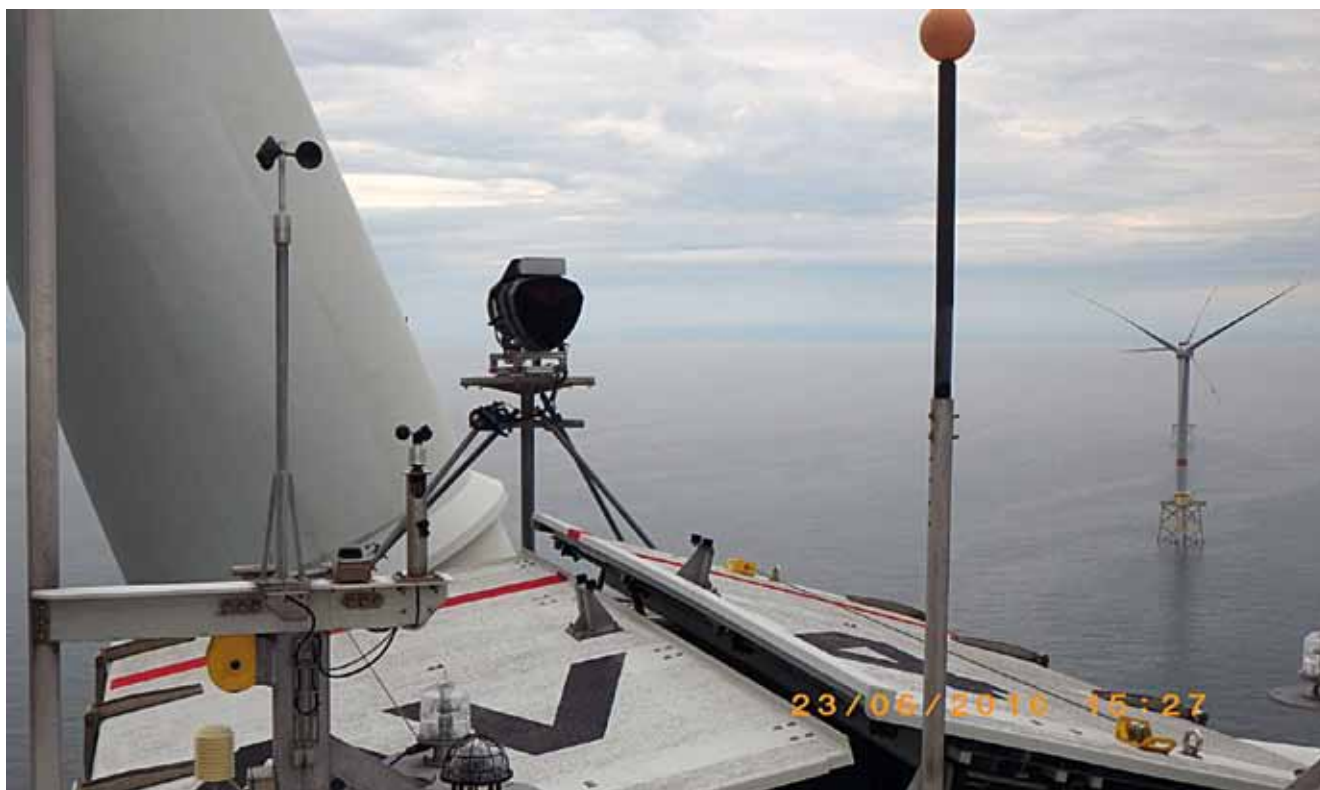
Figure 1: Free field test of short-range LiDAR System on top of Nacelle wind turbine AV04
