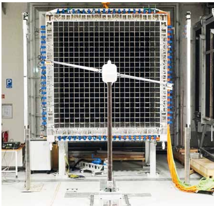
Figure 1: Model wind turbine of the Delft University of Technology in front of 3 m x 3 m active grid in the WindLab wind tunnel
