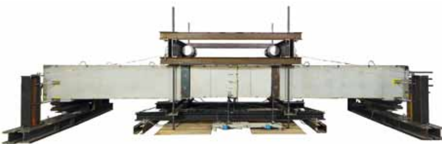
Figure 3: Set up of large-scale fatigue tests (© Institute of Concrete Construction)
