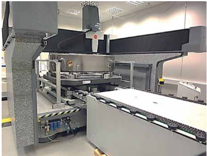
Figure 1: Coordinate measuring machine measuring the large gear standard
