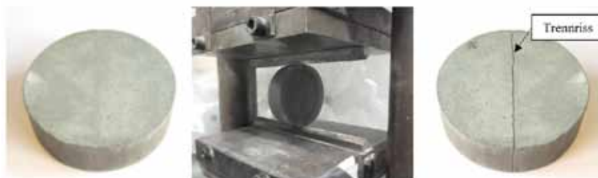
Figure 33: Implementation of cracks in specimens.
