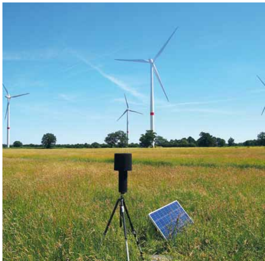
Figure 3: Acoustic measurement station to monitor wind turbine noise
