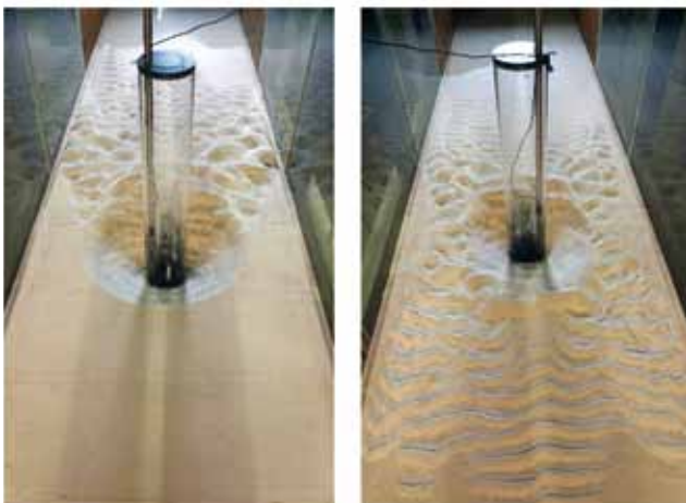
Figure 29: left: scour development after approx. 8 h with a unidirectional flow load of u = 0.2 \text{ m/s} ; right: scour development after approx. 8 h as a result of tidal flow with a maximum flow velocity (peak) of u = 0.25 \text{ m/s}
