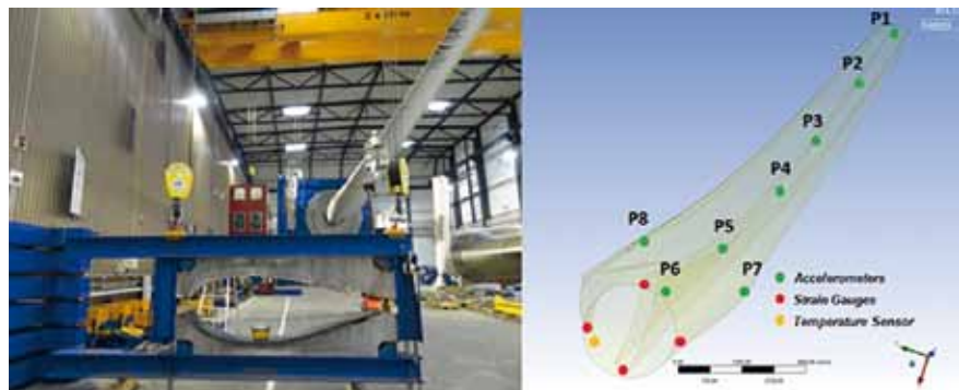
Figure 2: Fatigue test on a 34 m rotor blade and instrumentation
