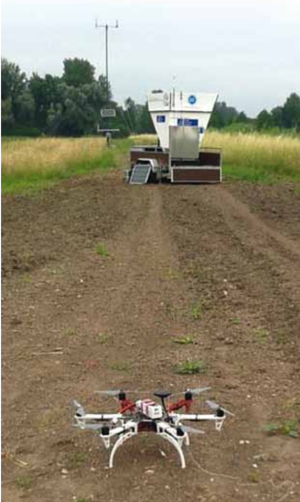
Figure 5: Multicopter and sodar to measure vertical wind-profiles
