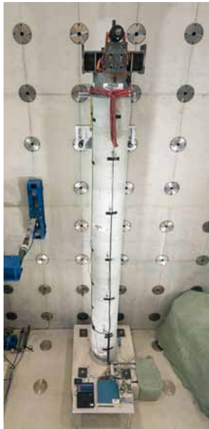
Figure 4: Pre-stressed concrete support structure equipped with accelerometers in a laboratory setup
