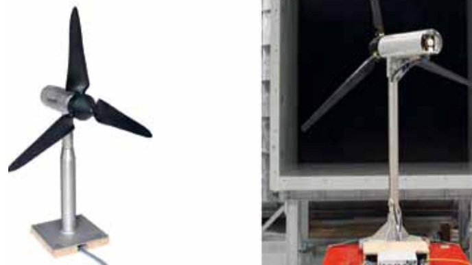
Figure 2: Left: Model wind turbine Oldenburg (MoWiTO 0.6) with a diameter of 0.58m. Right: Model wind turbine Oldenburg (MoWiTO 1.8) with a diameter of 1.8m. Pictures are not in scale.
