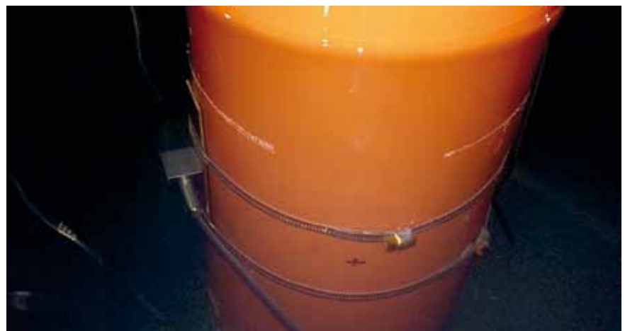
Figure 8: Application of damage to experimental pile
