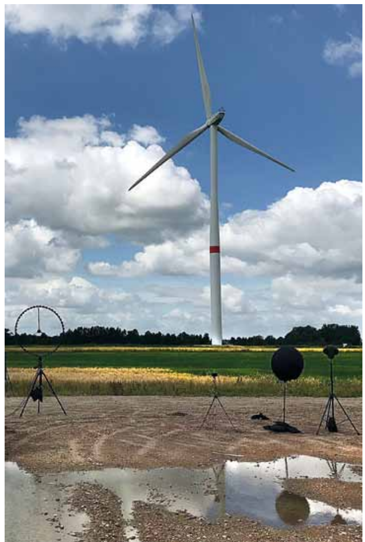
Figure 6: Measurement setup for the psychoacoustic evaluation of wind turbine noise
