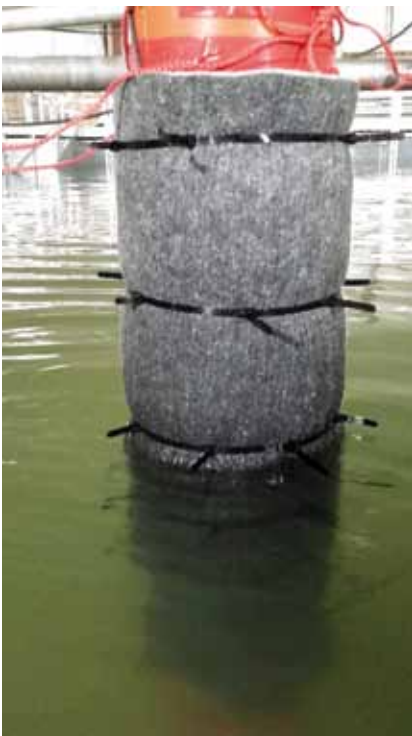
Figure 7: Application of synthetic sheets as marine growth
