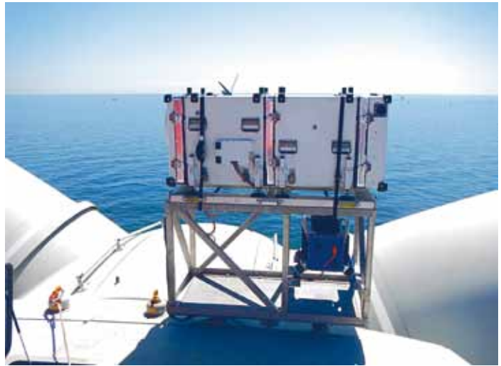
Figure 2: The robust and cost-efficient lidar system "Whirlwind 1" in the laboratory (left) and mounted offshore on AV07 in the alpha ventus wind farm, together with the SWE scanning lidar (right)
