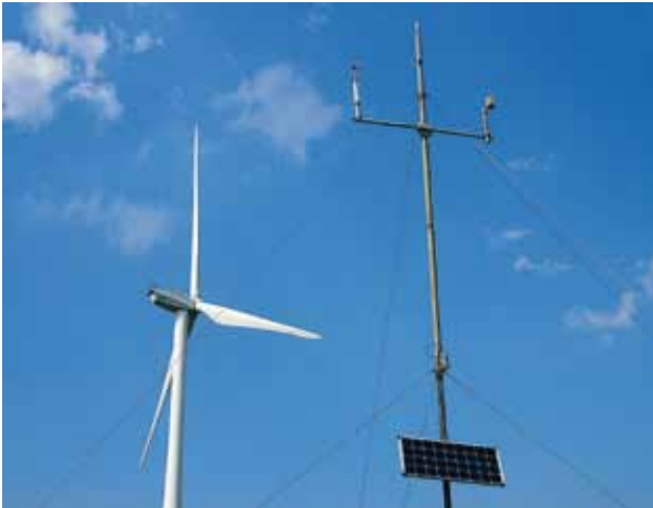
Figure 4: Mast for long-term measurement of wind speed and direction, temperature and humidity
