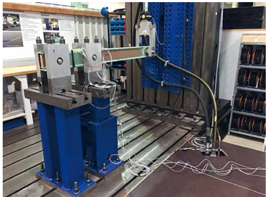
Figure 2: Test stand for beam samples at Fraunhofer IWES in Bremerhaven. A hydraulic actuator is applying force time series to the right end of the beam.
