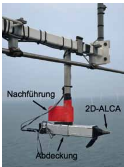
Figure 1: The 2D-ALCA mounted at the metmast of the FINO3-platform.
