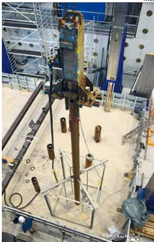
Figure 1: Photo of the test pit and the installed piles
