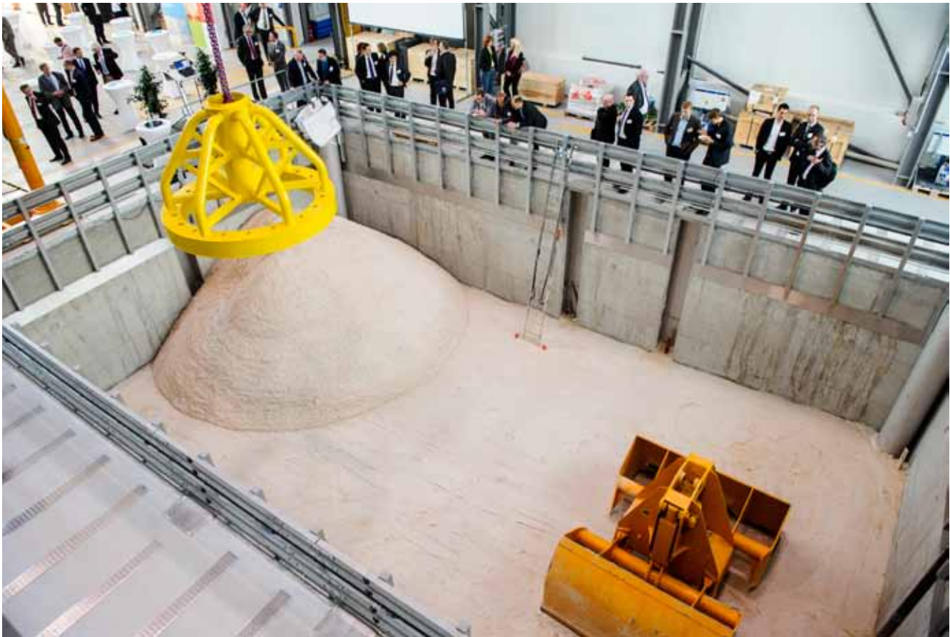
Foundation test pit of the Test Center, picture: Mathias Schumacher, Leibniz Universität Hannover
