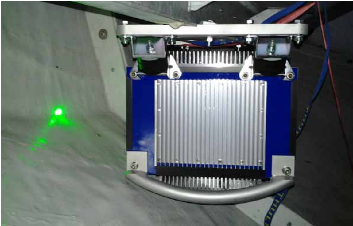
Figure 2: Experimental integration of Whirlwind 1 into the spinner of an AREVA Multibrid M5000 wind turbine, November 2013.
