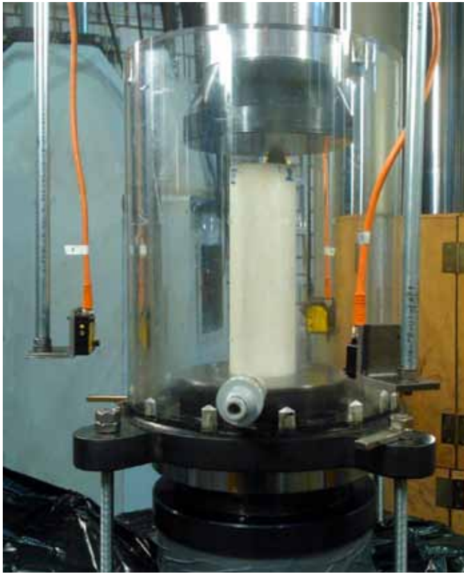
Figure 1: Under water test rig (Foto © Institute of Building Materials Science)
