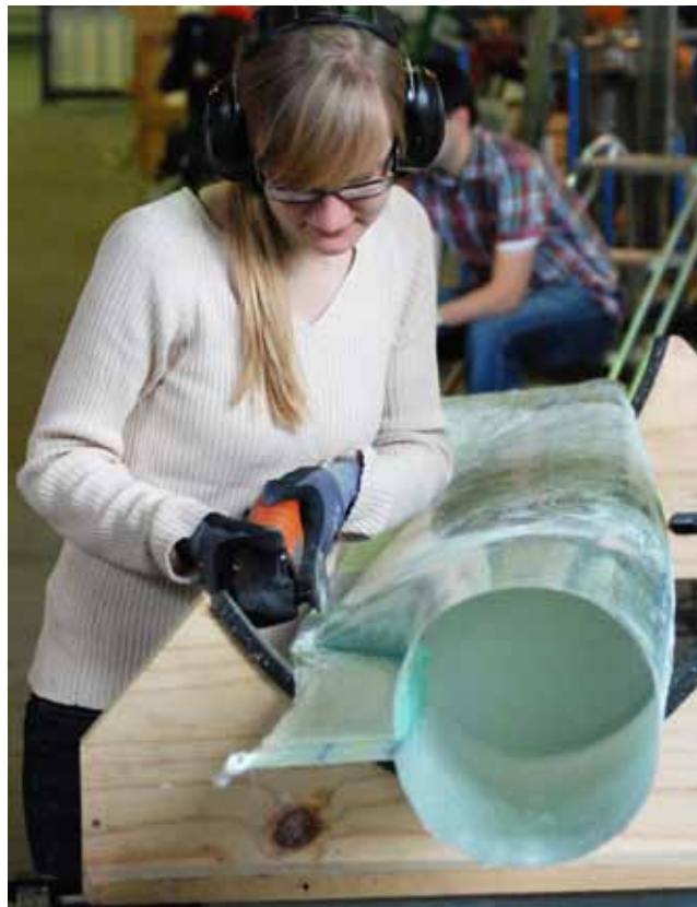
Figure 1: Student trimming the trailing edge of the small rotor blade model laminated during the Composite Lab (picture provided by Daria Horte, 2012).
