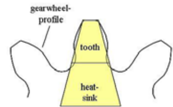
Figure 1: Model geometry of a tooth with a heat sink which presents the center of the gear wheel
