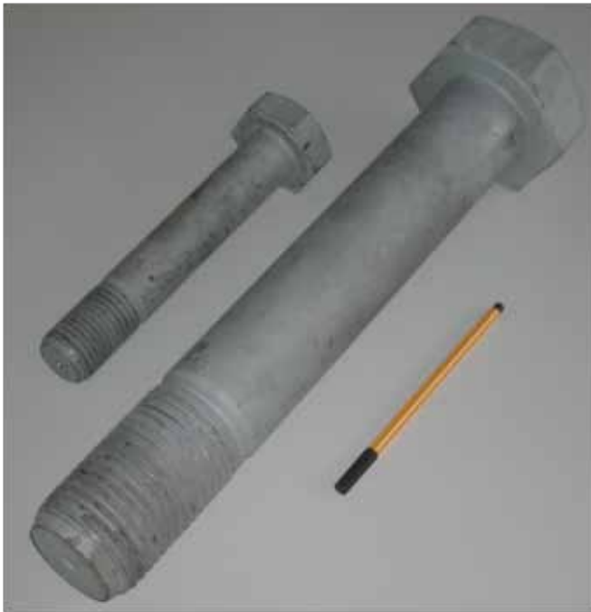
Figure 1. Hot-dip galvanized bolts M36 and M64
