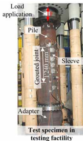
Figure 2: Large scale test specimen in testing facility
