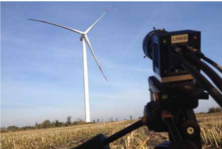
Figure 1: Field test for measuring rotor blade deformations with new optical measurement system
