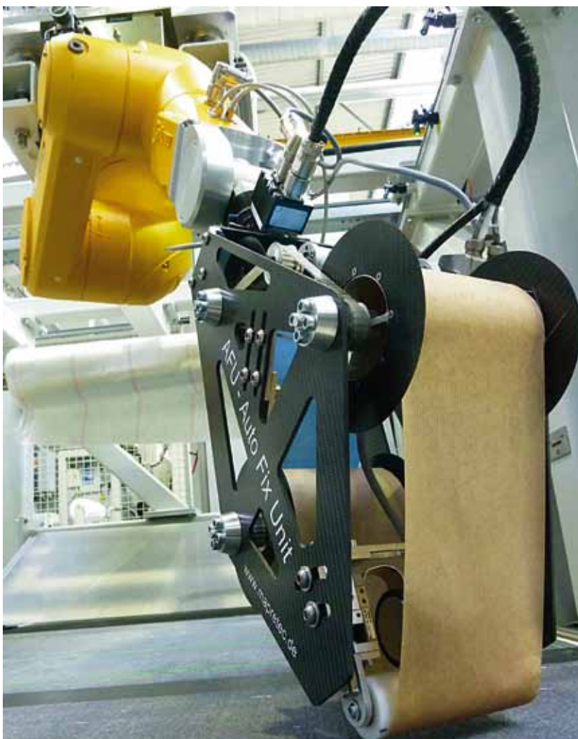
Figure 3: Auto Fix Unit mounted to the articulated arm
