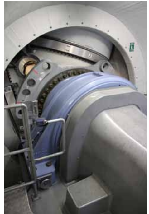
Figure 2: Rotor head and shaft of a wind energy system (Source: BIMAQ)
