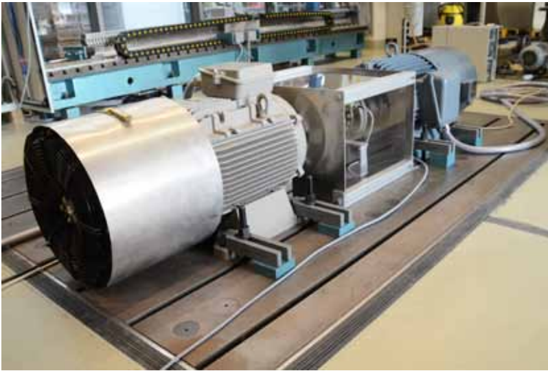
Figure 2: Test bench with synchronous generator (30 kW) and induction motor (45 kW) as drive
