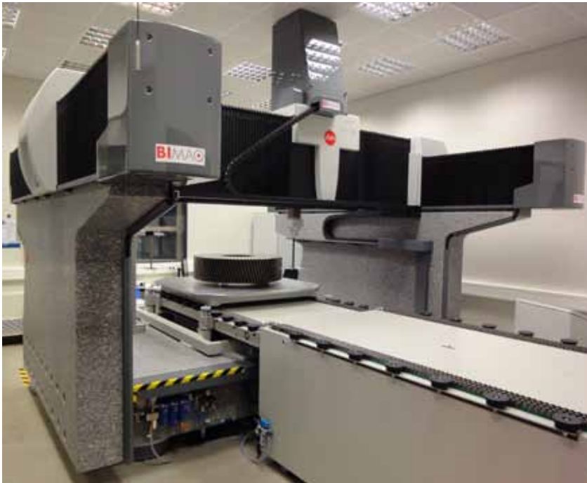
Figure 1: Leitz PMM-F 30.20.7 coordinate measuring machine at the Laboratory for large-scale gear-measurements (Source: BIMAQ)
