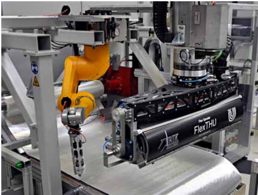
Figure 2: Material supply unit with ultrasonic cutter system and adaptive handling unit
