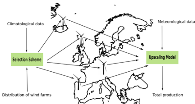
Figure 3: Selection of reference sites and an appropriate upscaling model is required to monitor European wind power adequately.
