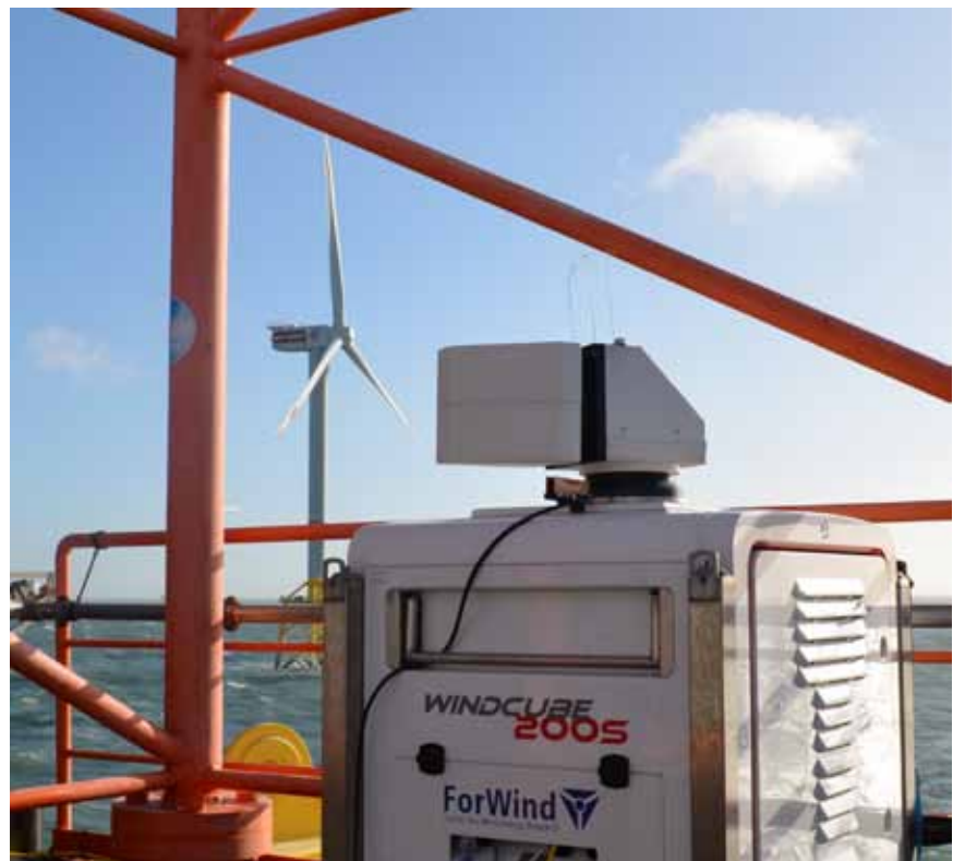
Figure 1: One of ForWind's long range scanning Lidars Windcube 2005 located on the offshore research platform Fino1 scanning the flow around a wind turbine in the nearby offshore wind farm »alpha ventus«.
