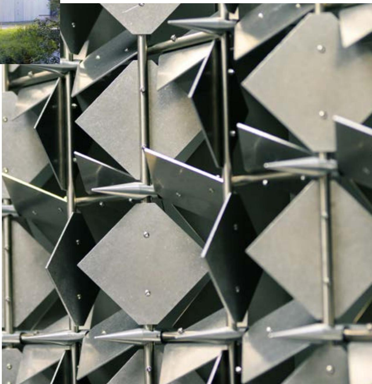
With the help of the turbulent wind tunnel, the ForWind scientists can downscale characteristics of complex atmospheric wind fields and thus reproduce characteristic properties of a real wind field in the wind tunnel. The goal is to investigate turbulent flows and their effects on the components and performance of wind turbines.
